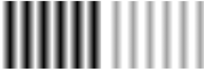
Figure 3-3: Typical Sine Wave Gratings for Testing Contrast.
